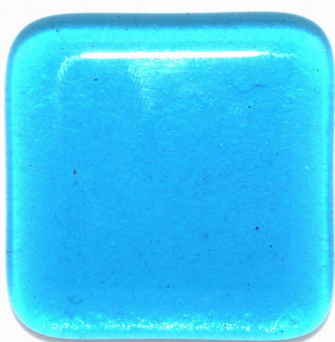
2 layers, total 6 mm No loss of shape, nicely rounded edges
