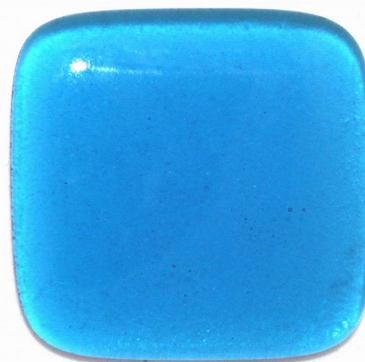
3 layers, total 9 mm Size has grown and shape has "blown up"
