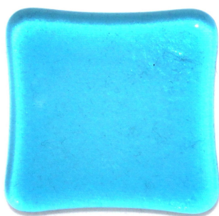
1 layer, total 3 mm The glass was pulled inwards
